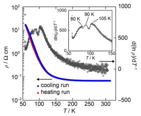
Fig. 2 Temperature dependence of the resistivity ( $\rho$ , blue and red lines) and the derivative of the resistivity  $(d(\ln \rho)/d(T^{-1}))$ , black circle) of (1)PF<sub>6</sub> at a heating run
