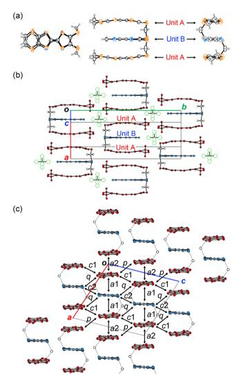
Fig. 3 (a) Molecular structures (top, side, and end views) of 1, (b) crystal structure viewed along the donor short axis, and (c) conducting sheet viewed along the donor long axis in (1)PF<sub>6</sub> at 296 K. Hydrogen atoms in (c) are omitted for clarity
