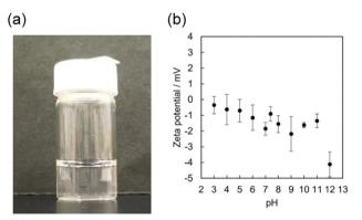
Fig. 2 (a) Image of  $\gamma$ -CyDng agueous solution (100 mg mL<sup>-1</sup>). (b) Zeta potentials of  $\gamma$ -CyDngs in water (5 mM HEPES buffer) under various pH conditions (n = 5) at 25 °C.
