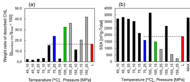
Fig. 2 (a) Weight ratio of desorbed CHL during the TG measurement. (b) SSA after the impregnation processes. L: Liquid impregnation process, MAX: Maxisorb<sup>®</sup>.
