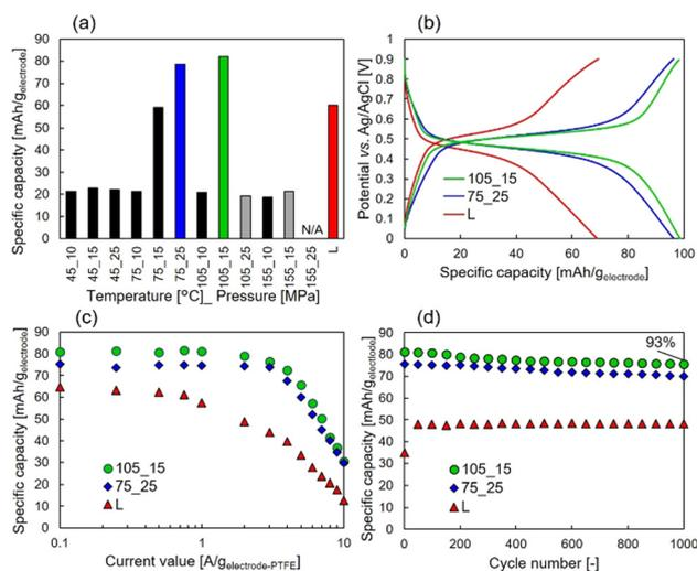
Fig. 3 (a) Specific capacity of each sample at  $0.1 \text{ A g}_{\text{electrode-PTFE}}^{-1}$ . (b) Constant current measurements for two  $\text{scCO}_2$  impregnated and liquid-impregnated samples with  $1 \text{ A g}_{\text{electrode-PTFE}}^{-1}$  of current density. (c) Rate characteristics of the three samples. (d) Cycle characteristics for two samples.
