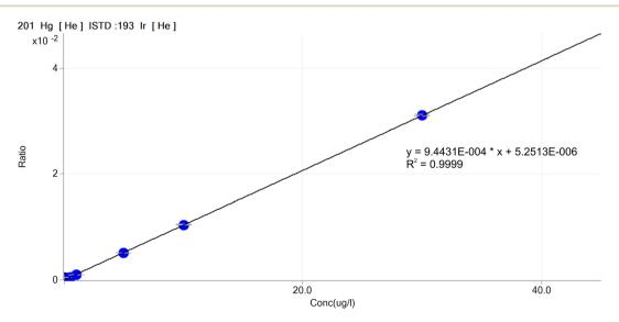
Fig. 1 Calibration curve used for mercury analysis. Calibration solutions were prepared with diluent A. Acquisition was conducted in He mode with internal standardization.
