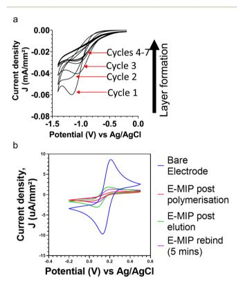
Fig. 1 (a) Layer by layer deposition of pNHMA E-MIP on BT-Au SPE vs. Ag/AgCl reference electrode using cyclic voltammetry (-0.2 V and -1.4V vs. Ag/AgCl reference; 7 cycles at 50 mV s<sup>-1</sup>). (b) CV of ferro/ferricyanide redox marker at different stages of electrode modification: bare (blue); post E-MIP polymerisation (red); post template, BHb elution (green); and after 5 min of template, BHb (1 nM) rebinding (purple).
