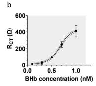
Fig. 6 Standard curve for BHb determination using BHb MIP-modified BT-Au electrode (a), (b) Shows linear range in (a) expanded, Saturation occurs at 1 nM of target protein, indicating that all MIP cavities are occupied with protein. KD was determined to be 0.86 + 0.11 nM using the Hill-Langmuir method. Data represents mean + S.E.M., n = 3.
