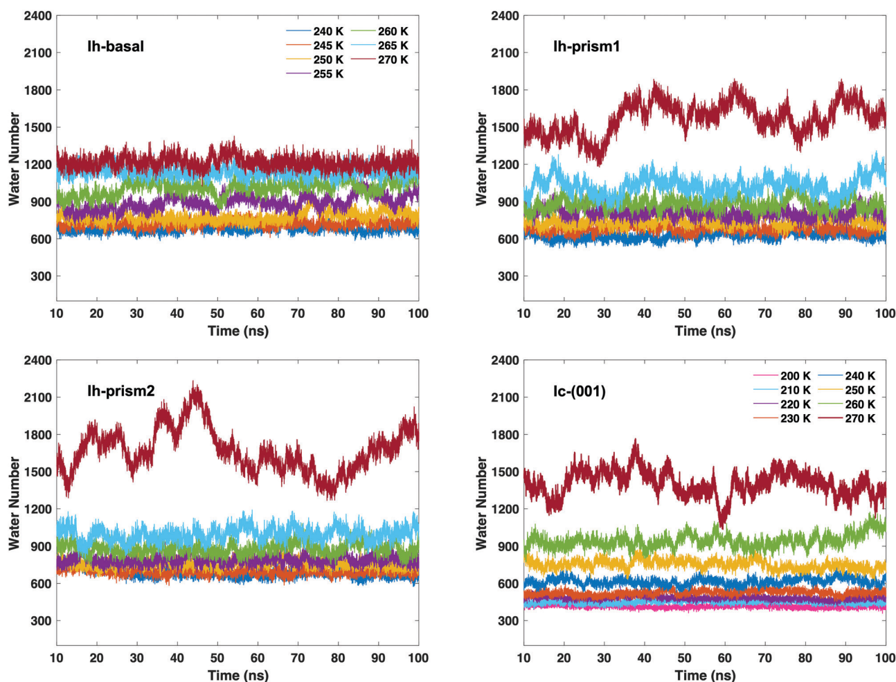
Fig. 4 Time-evolution of the number of liquid-like molecules in QLLs on the basal (top-left panel, with temperature legend for Ih), prism1 (top-right panel), and prism2 (bottom-left panel) surfaces of Ih in the 240–270 K range of temperature and on the (001) surface of Ic (bottom-right panel, with temperature legend for Ic) in the 200–270 K range of temperature, using the local entropy fingerprint le as order parameter.
