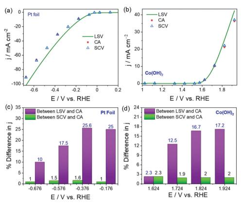
Fig. 4 (a) HER polarization curves of Pt foil acquired using LSV and SCV and provided in comparison with CA data. (b) OER polarization curves of Co(OH)<sub>2</sub> acquired using LSV and SCV and provided in comparison with CA data. (c and d) The plots of % difference in j between LSV and CA, and SCV and CA against potential showing the closeness of SCV and CA. Reproduced from ref. 64 (Copyright 2022, IOP Publishing)
