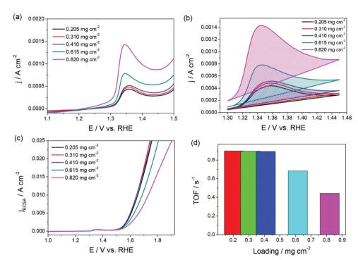
Fig. 1 (a and b) LSVs of NiO/GC showing the oxidation of NiO to NiOOH with increasing loading. (c and d) Relative specific activity and TOF of the same showing loading independence until the surface coverage exceeded 100%. Reproduced from ref. 68 (Copyright 2019, American Chemical Society).
