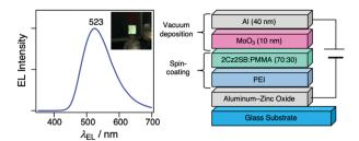
Fig. 7 An EL spectrum and device structure of the solution-processed OLED containing 2Cz2SB. (Inset: Photograph of OLED upon application of external voltage of 5 V).
