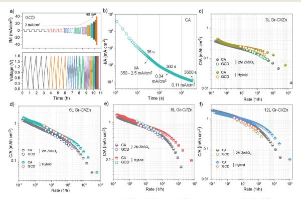
Fig. 5 Comparison of capacity-rate data using conventional GCD and CA method. (a) Rate measurements of 3D Gr-C//Zn cell analysed using conventional GCD tests (bottom) with increasing charge-discharge I/A of 3 to 40 mA cm<sup>-2</sup> (top). (b) I/A transient as a function of time obtained via the CA method for 12L 3D Gr-C//Zn cell. (c-f) comparison of capacity vs. rate curves obtained via CA and GCD methods using 3-12L printed Gr-C//Zn cells in pristine ZnSO<sub>4</sub> and hybrid electrolytes.
