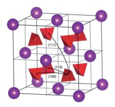
Fig. 12 Locally relaxed average crystal structure of  $\delta$ -Bi<sub>2</sub>O<sub>3</sub>, where the purple spheres represent Bi atoms and the red tetrahedra represent disordered O positions. Black arrows indicate possible oxygen jumps in (100), (110), and (111) directions. Adapted from ref. 95.
