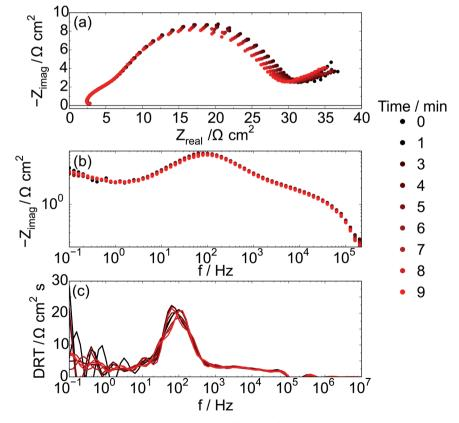
Fig. 7 Impedance spectra recorded during the strongest polarization (85%  $I_{\text{max}}$ /5.5 mA) of the Ni-Co-CGO cell in 100% CH<sub>4</sub> at 750 °C; (a) plotted as Nyquist plots and (b) plotted as Bode plots, (c) DRT representation.
