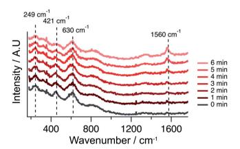
Fig. 8 Raman spectra recorded during the strongest polarization (85%  $I_{\rm max}$ ) of the Ni–Co–CGO cell in 100% CH<sub>4</sub> at 750 °C. Notably, the spectra are vertically shifted for clarity.
