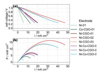
Fig. 3 Initial LSV (a) and power density curves (b) of all the tested cells, measured in 3% H<sub>2</sub>O/H<sub>2</sub> at 750 °C
