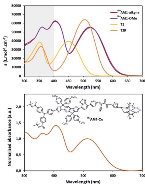
Fig. 3 UV-Vis spectra of dyes <sup>t</sup>BuAM1-alkyne, <sup>t</sup>BuAM1-OMe, <sup>t</sup>BuT1 and <sup>t</sup>BuT2R (top) and dyad <sup>t</sup>BuAM1-Co (bottom), recorded in DCM at 25 °C.
