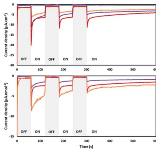
Fig. 4 Top: Chopped-light chronoamperometric measurements recorded at +0.14 V vs. RHE in 0.1 M aqueous MES/NaCl buffer pH 5.5 on a NiO (grey line), a NiO|**AM1-OMe** (purple line), a NiO|**AM1-Co** (red line) and a 1.5% Li-NiO|**AM1-Co** (orange line) photocathodes. Bottom: Normalized photocurrent densities related to the loading in photoactive component.
