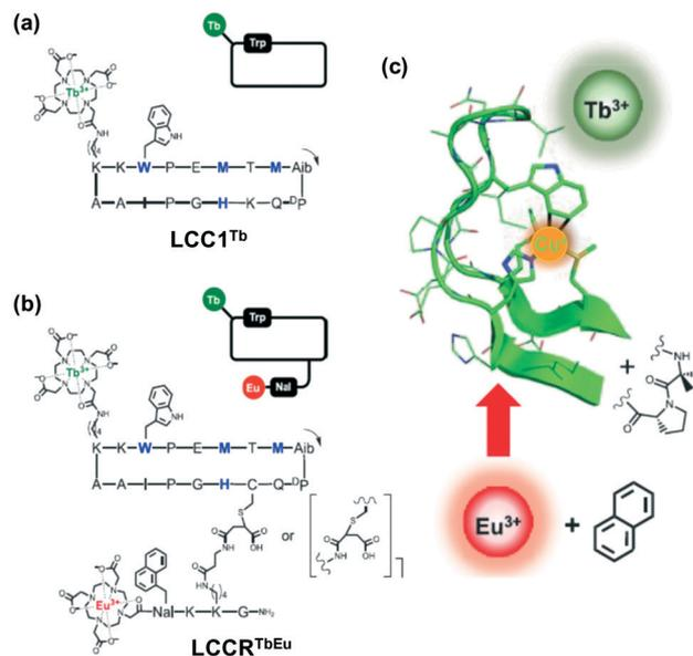
Fig. 28 Chemical structure and schematic representation of (a) **LCC1<sup>Tb</sup>** and (b) **LCCR<sup>TbEu</sup>**, Cu-chelating amino acids in blue and black. The arrow indicates the N-to-C direction within the cyclic peptide. Nal = 3-(1-naphthyl)-L-alanine; Aib = 2-aminoisobutyric acid; DP = D-proline. (c) Cu<sup>+</sup> binding site of CusF and design principle showing the positioning of the various components. Adapted from ref. 123.
