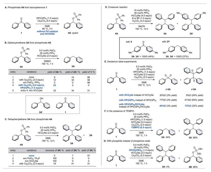
Fig. 3 (A) Phosphinate 4A from benzophenone (1). (B) Diphenylmethane (2A) from phosphinate 4A. (C) Tetraphenylethane 3A from phosphinate 4A. (D) Crossover reaction. Numbers in the parentheses are yields of 3A. (E) Deuterium labeling experiments. (F) Standard conditions with TEMPO as a radical scavenger. (G) With phosphite instead of phosphine oxide.
