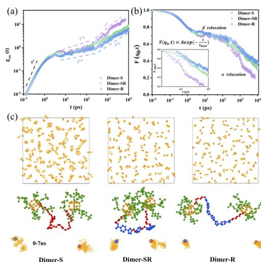
Fig. 4 MD simulations for dimer molecules (64 dimer molecules in the bulk). (a) Mean square displacement of center-of-mass of OPOSS,  $g_{\text{cm}}(t)$ , of different dimers. (b) The self-part of the intermediate scattering function of different dimers. (c) Center-of-mass motion trajectories of OPOSS of different dimers from 0 to 7 ns.
