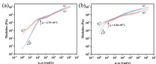
Fig. 2 Master curves constructed from SAOS data from 273 K to 323 K. (a) Dimer-SR and (b) Dimer-R at a reference temperature of 323 K. The horizontal shifting factor  $a_T$  of dimer molecules and OPOSS collected from time–temperature superposition of the small-amplitude oscillatory shear (SAOS) data (Fig. S6†). The relationship between  $a_T$  and  $1/T$  is well established by fitting to the WLF formula as is shown in Fig. S9.†
