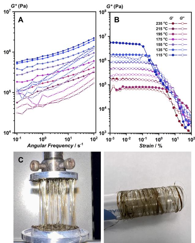
Fig. 3 (A) Frequency sweep and (B) strain sweep viscoelastic measurements of **1** from 235 to 115 °C under N<sub>2</sub> flow. (C) Fibers of **1** prepared by a melt-quench process by use of hot press and collected by spinning around the glass tube.
