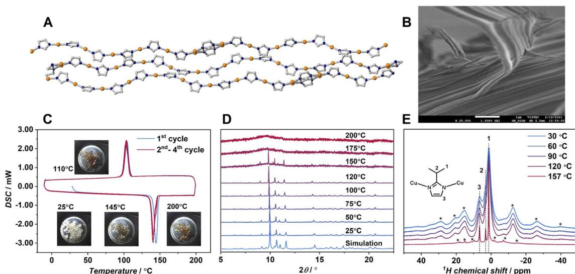
Fig. 1 (A) Crystal structure. Cu: orange; C: gray; N: dark blue and (B) SEM image of **1**. Isopropyl groups are omitted. (C) DSC profiles on the first cycle (sky blue) and the second to fourth cycles (red) of **1**. 10 K min<sup>-1</sup> under N<sub>2</sub> flow. (D) VT-PXRD of **1**. Wavelength was  $\lambda = 0.99998$  Å. (E) <sup>1</sup>H magic-angle spinning solid-state NMR of **1** at temperatures of 30, 60, 90, 120, and 157 °C. Asterisk denotes spinning sidebands.
