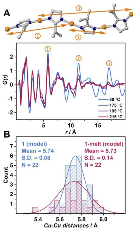
Fig. 2 (A) Partial crystal structure of **1** showing the intrachain Cu–Cu correlations at approximately ① 6.10, ② 11.6, ③ 17.1 Å and radial distribution function of **1** at 30 °C and **1-melt** at 175, 195 and 215 °C. (B) Distribution plots of Cu–Cu distances of **1(model)** (blue) and **1-melt(model)** (red) generated from MD simulation. S.D. is the standard deviation, and  $N$  is the number of the population.
