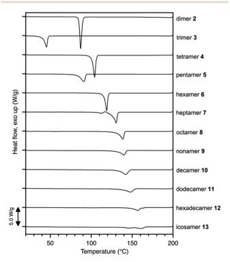
Fig. 4 DSC traces (1st heating run) of discrete oligomers 2–13 at 10  $^{\circ}$ C min<sup>-1</sup>.
