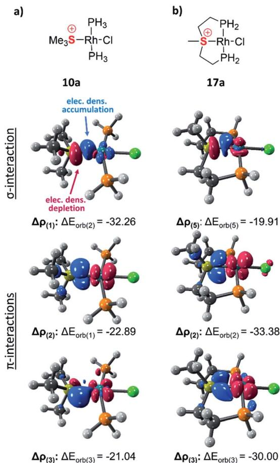
Fig. 5 Selected deformation density plots of model complexes **10a** (a) and **17a** (b) (all energies are given in kcal mol<sup>-1</sup>).
