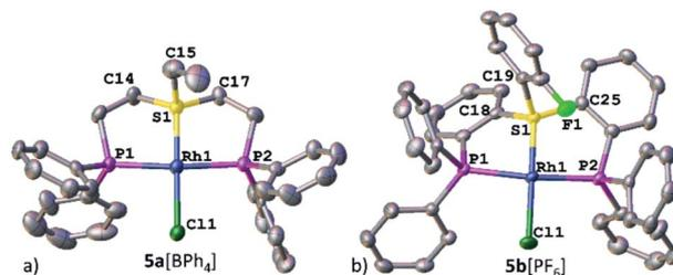
Fig. 3 XRD structures of Rh(I)-sulfonium complexes,  $5\text{a}[\text{BPh}_4]$  (a) and  $5\text{b}[\text{PF}_6]$  (b). Co-crystallized solvent molecules, counter anions, and hydrogen atoms are omitted for clarity.
