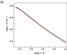
Fig. 5 (a) Current–voltage (I-V) characteristics of PMC-hexagon in three different pellets at RT. (b) Temperature dependence of the electrical conductivity  $(\sigma)$  of PMC-hexagon fitted with the Arrhenius equation (red line).
