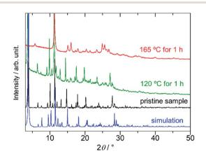
Fig. 3 Powder X-ray diffraction (PXRD) patterns of PMC-hexagon (simulated from the crystal structure: blue, pristine sample: black, heated at 120  $^{\circ}$ C for an hour: green, and heated at 165  $^{\circ}$ C for an hour: red).
