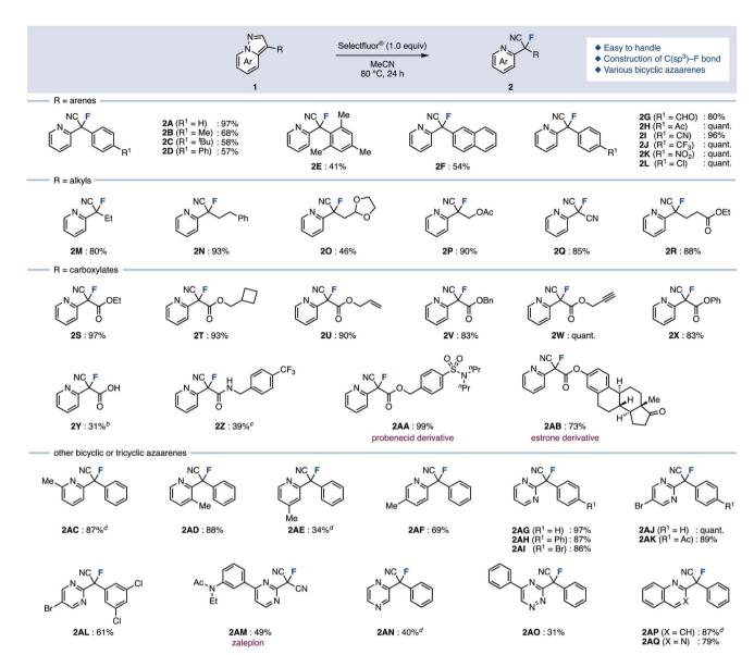
Scheme 1 Substrate Scope. <sup>a</sup> Conditions. 1 (0.20 mmol), Selectfluor® (1.0 equiv.), MeCN (1.0 mL), 80 °C, 24 h. <sup>b</sup> Selectfluor® (5.0 equiv.) was added. <sup>c</sup> The reaction was performed at -30 °C. <sup>d</sup> NaClO<sub>4</sub> (1.0 equiv.) was added.
