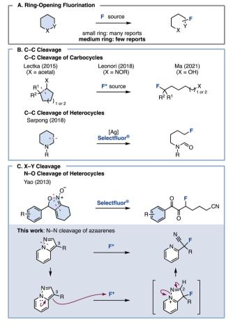
**Fig. 1** (A) Ring-opening fluorination. (B) Fluorination of cyclic compounds *via* C–C bond cleavage. (C) Fluorination of cyclic compounds *via* X–Y bond cleavage.
