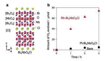
Fig. 1 (a) Crystal structure of the layered perovskite oxyhalide Bi<sub>4</sub>-NbO<sub>8</sub>Cl. (b) Time courses of H<sub>2</sub> evolution over Bare-Bi<sub>4</sub>NbO<sub>8</sub>Cl (squares), Rh-Bi<sub>4</sub>NbO<sub>8</sub>Cl (triangles) and Pt-Bi<sub>4</sub>NbO<sub>8</sub>Cl (circles) in a methanol aqueous solution (20 vol%) under photoirradiation ( $\lambda$  > 300 nm).
