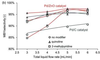
Fig. 4 The effect of selected catalyst modifier on (a) conversion and (b) selectivity in MBY semi-hydrogenation over the (black) Pd/C and (red) Pd/ ZnO catalysts.
