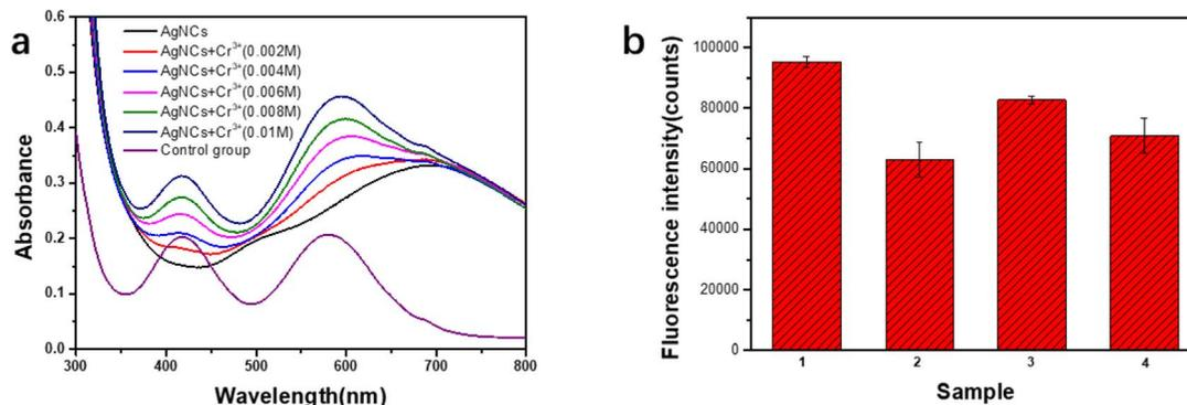
Fig. 7 (a) UV-vis spectra and fluorescence spectra of PAA-AgNCs with different components (control: PAA, isopropanol and  $\text{Cr}^{3+}$  ions); (b) fluorescence intensity of PAA-AgNCs after  $\text{Cr}^{3+}$  ions addition under different conditions (1: AgNCs; 2: AgNCs and  $\text{Cr}^{3+}$  ions; 3: AgNCs,  $\text{Cr}^{3+}$  ions and PAA (add at the same time); 4: AgNCs,  $\text{Cr}^{3+}$  ions and PAA (add after fluorescence quenching)).
