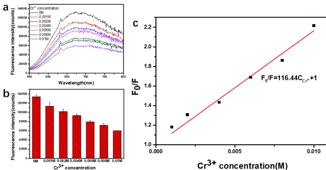
Fig. 6 (a) Fluorescence spectra of PAA-AgNCs with different concentrations of Cr<sup>3+</sup> ions; (b) the relationship between the fluorescence intensity of PAA-AgNCs and the concentration of Cr<sup>3+</sup> ions; (c) Stern-Volmer fluorescence quenching curve.
