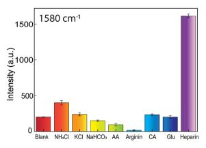
Fig. 12 Selectivity study of the AuNFs-4-MBA@chitosan SERS-tag nanoprobe. Comparison of the SERS peak intensity of 4-MBA at 1580 cm $^{-1}$  after adding different substances, involving 50 ppm heparin,  $10^{-2}$  M KCl,  $10^{-4}$  NaHCO3,  $10^{-4}$  M NH4Cl,  $10^{-4}$  M ascorbic acid (AA),  $10^{-4}$  M arginine,  $10^{-4}$  M citric acid (CA), and  $10^{-6}$  M glucose substances.
