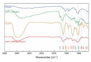
Fig. 8 FTIR spectrum of pure chitosan, AuNF-chitosan, pure heparin, and as-prepared AuNF-chitosan-heparin.
