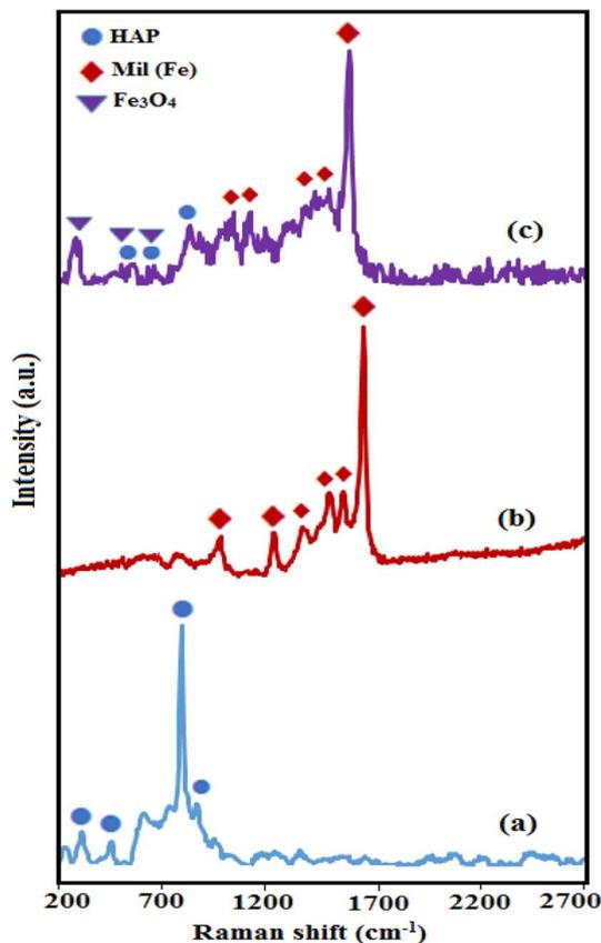
Fig. 3 Raman spectra of (a) pure HAP, (b) MIL-101(Fe) and (c) HAP/MIL-101(Fe)/Fe<sub>3</sub>O<sub>4</sub> nanocomposite.
