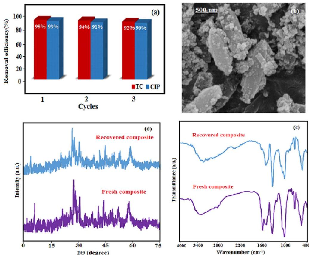
Fig. 14 (a) Reusability of the HAP/MIL-101(Fe)/Fe<sub>3</sub>O<sub>4</sub> nanocomposite in the removal of TC and CIP antibiotics, (b) SEM image, (c) FT-IR spectrum and (d) XRD patterns of the fresh and recovered nanocomposite after three runs.
