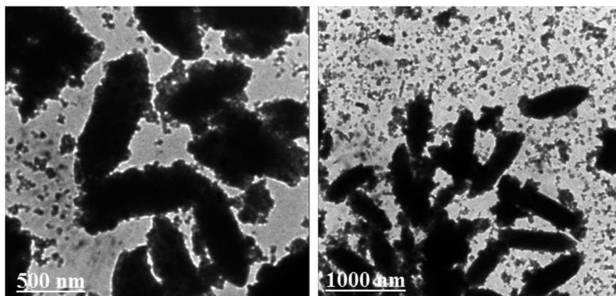
Fig. 5 TEM images of the HAP/MIL-101(Fe)/Fe<sub>3</sub>O<sub>4</sub> nanocomposite.
