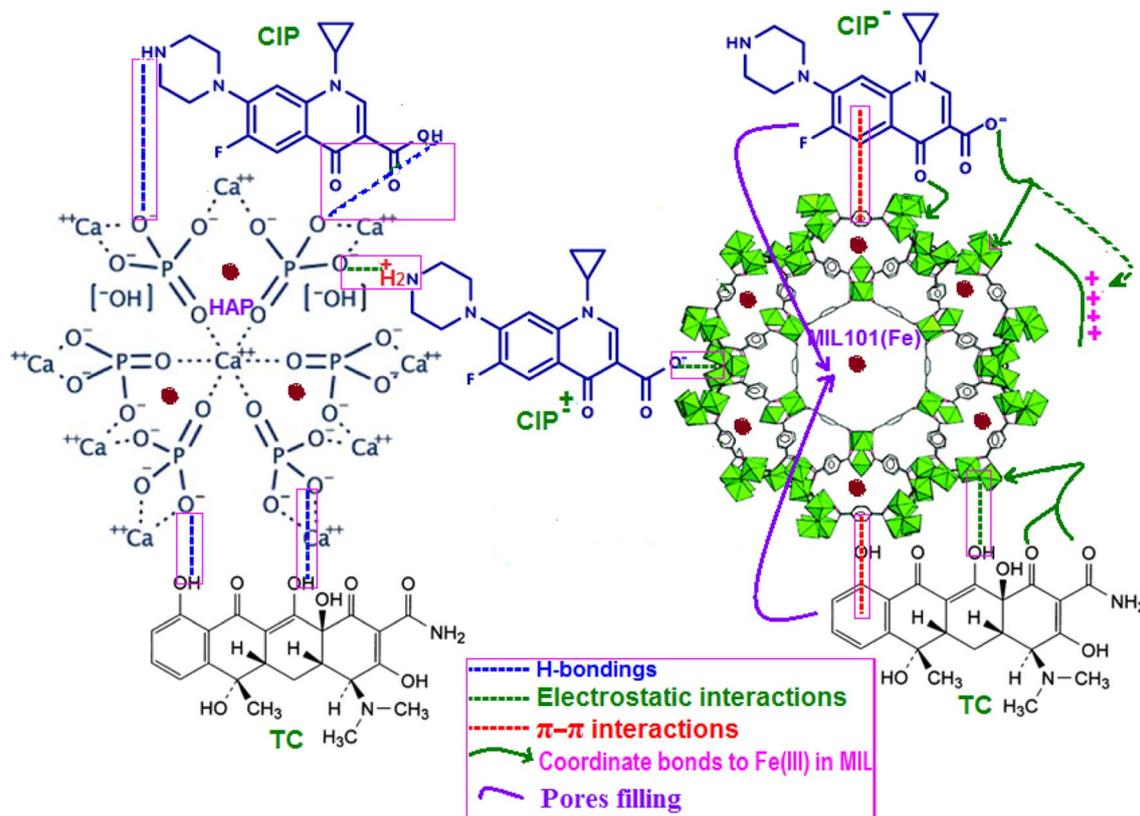
Fig. 13 Schematic diagram of the suggested adsorption mechanism of TC and CIP on HAP/MIL-101(Fe)/Fe<sub>3</sub>O<sub>4</sub> nanocomposite.
