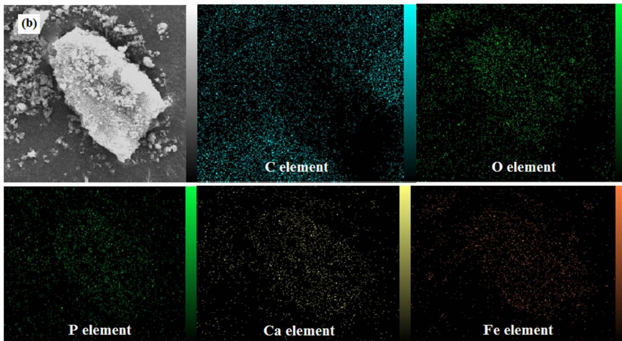
Fig. 6 (a) EDX spectrum and (b) elemental mappings of the HAP/MIL-101(Fe)/Fe<sub>3</sub>O<sub>4</sub> nanocomposite.
