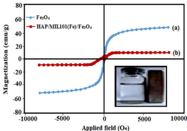
Fig. 7 Magnetization curves of (a) pure  $\text{Fe}_3\text{O}_4$  and (b) HAP/MIL-101(Fe)/ $\text{Fe}_3\text{O}_4$  nanocomposite at room temperature (inset: the magnetic separation of HAP/MIL-101(Fe)/ $\text{Fe}_3\text{O}_4$  nanocomposites by a magnet).
