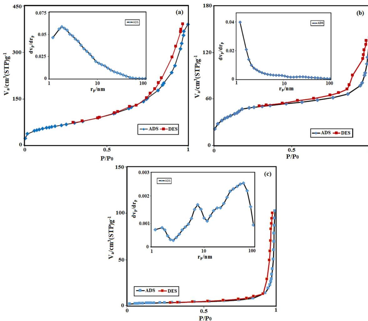
Fig. 8 Nitrogen adsorption–desorption isotherms of (a) pure HAP, (b) MIL-101(Fe) and (c) HAP/MIL-101(Fe)/ $\text{Fe}_3\text{O}_4$  nanocomposite. The insets show the corresponding pore size distribution curves.
