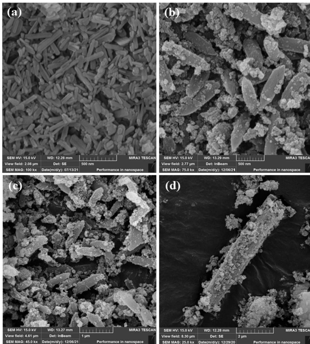
Fig. 4 (a) SEM image of pure HAP and (b)–(d) SEM images of the HAP/MIL-101(Fe)/Fe<sub>3</sub>O<sub>4</sub> nanocomposite.
