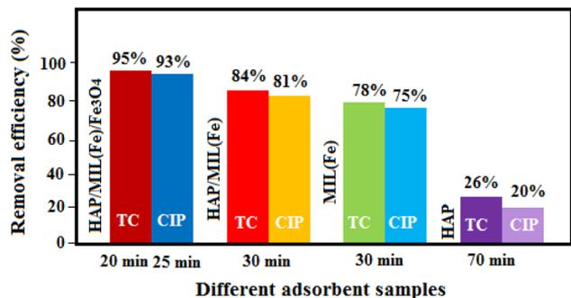
Fig. 12 Removal efficiency of the nanocomposite components.
