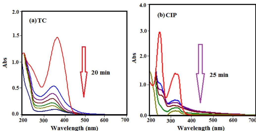
Fig. 10 UV-vis spectral changes of drugs aqueous solutions with HAP/MIL-101(Fe)/Fe<sub>3</sub>O<sub>4</sub> at different time intervals: (a) TC and (b) CIP (experimental conditions: [drug]<sub>0</sub> = 50 mg L<sup>-1</sup>, V = 50 mL, adsorbent dose: 30 mg at 25 °C).
