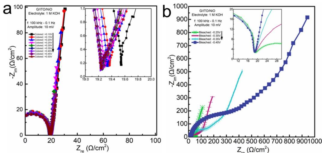
Fig. 6 EIS data and analysis for NiO thin films measured in 1 M KOH electrolyte: (a) gradual coloration applying increased magnitude potentials (+0.1 V, +0.5 V); (b) gradual bleaching range from  $(-0.25 \text{ V}, -0.4 \text{ V})$ .
