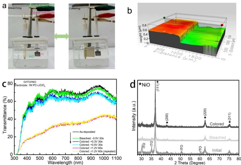
Fig. 1 (a) Electrochemical test setup; (b) surface imaging; (c) optical modulation of NiO thin solid film as deposited, in the bleached state and colored states; and (d) XRD patterns of initial/colored/bleached states.
