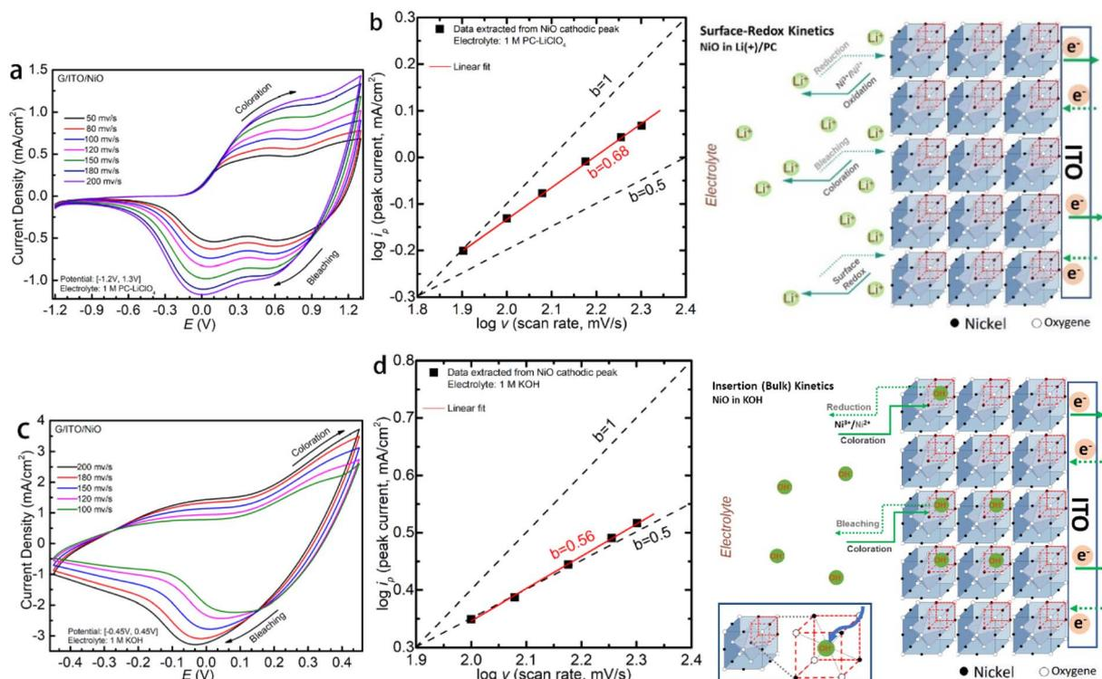
Fig. 3 (a and c) CV curves at different scan rates of NiO in Li-PC and KOH, respectively; (b and d) linear fitting of log *i*<sub>p</sub> vs. log *v* and proposed dominant electrochemical kinetics at the interface in Li-PC and KOH, respectively.
