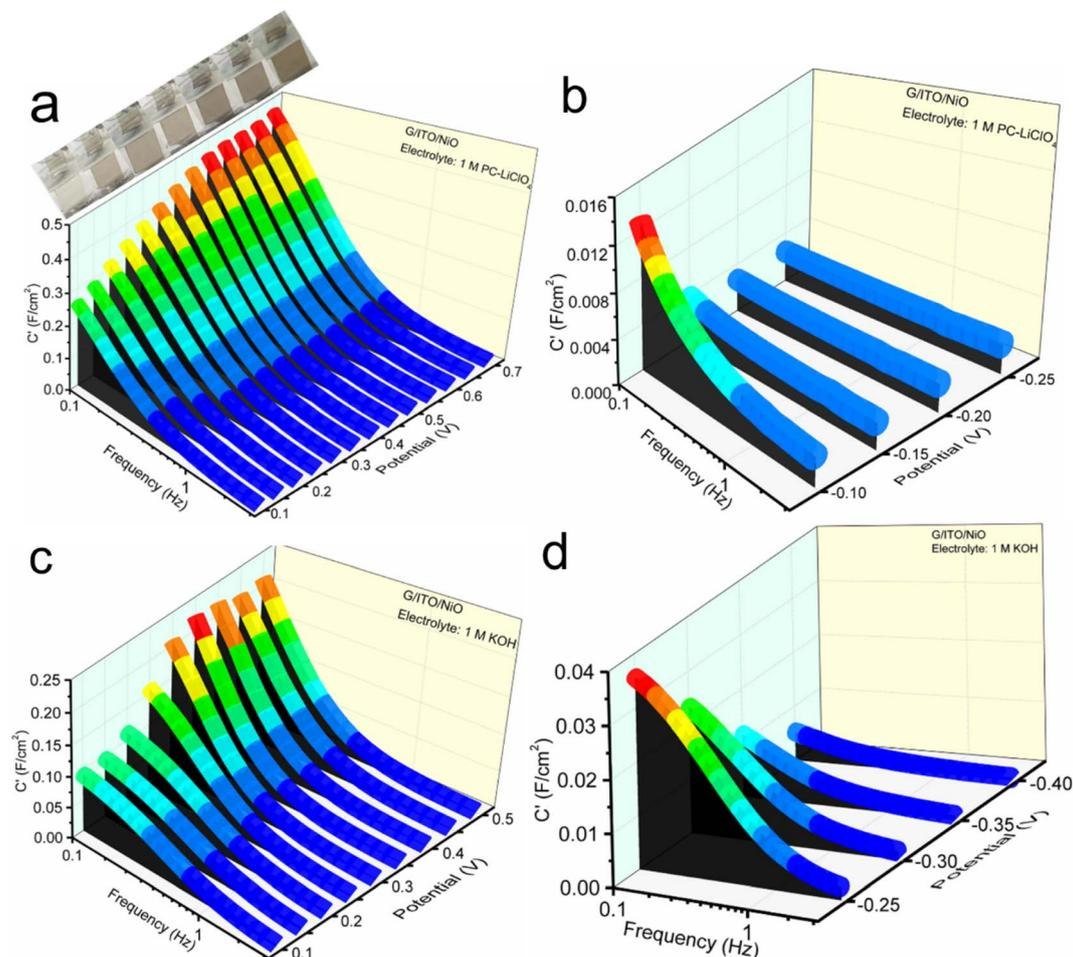
Fig. 8 The 3D Bode plot representations of the real capacitance  $C'$  vs.  $f$  vs. potential at firstly charging and then discharging states of NiO in (a and b) PC-Li<sup>+</sup> and (c and d) KOH electrolytes with potentials ranging from 0 up to 0.7 V.
