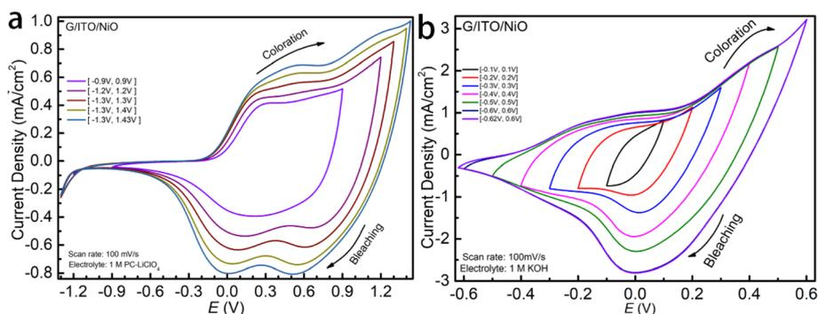
Fig. 2 (a and b) CV of NiO in 1 M LiClO<sub>4</sub>-PC and 1 M KOH as a function of potential windows.
