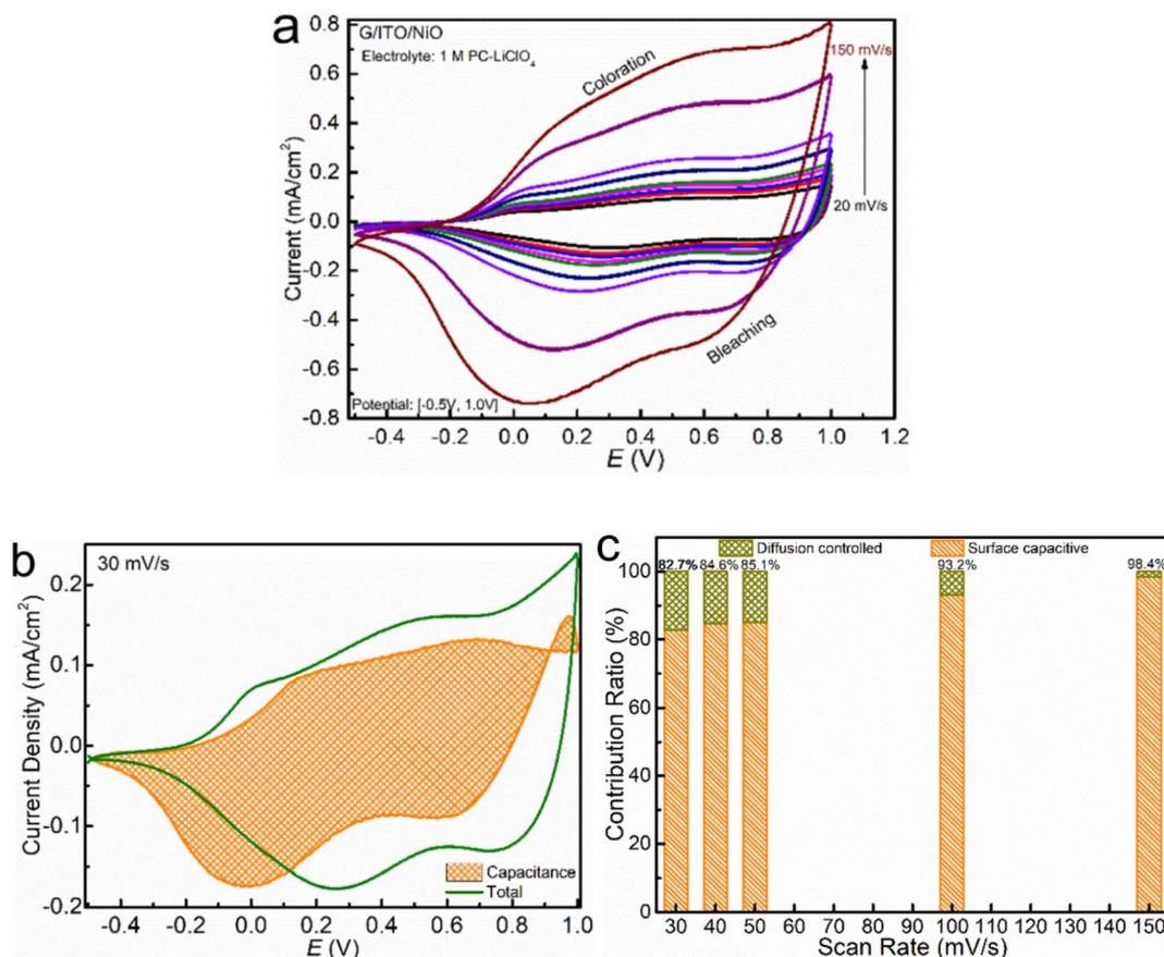
Fig. 9 (a) CV curves from 20 mV s<sup>-1</sup> to 150 mV s<sup>-1</sup> scan rates (b) CV curves at 30 mV s<sup>-1</sup> illustrating the surface capacitance contribution (shaded area) to the total. (c) Percentage of diffusion-controlled and surface capacitive behavior varying with scan rate.
