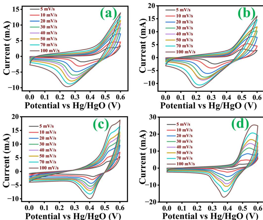
Fig. 6 Cyclic voltammograms at several scan rate of (a) Co<sub>3</sub>O<sub>4</sub>, (b) Co<sub>3</sub>O<sub>4</sub>@MnO<sub>2</sub>-1, (c) Co<sub>3</sub>O<sub>4</sub>@MnO<sub>2</sub>-2 and (d) Co<sub>3</sub>O<sub>4</sub>@MnO<sub>2</sub>-3.
