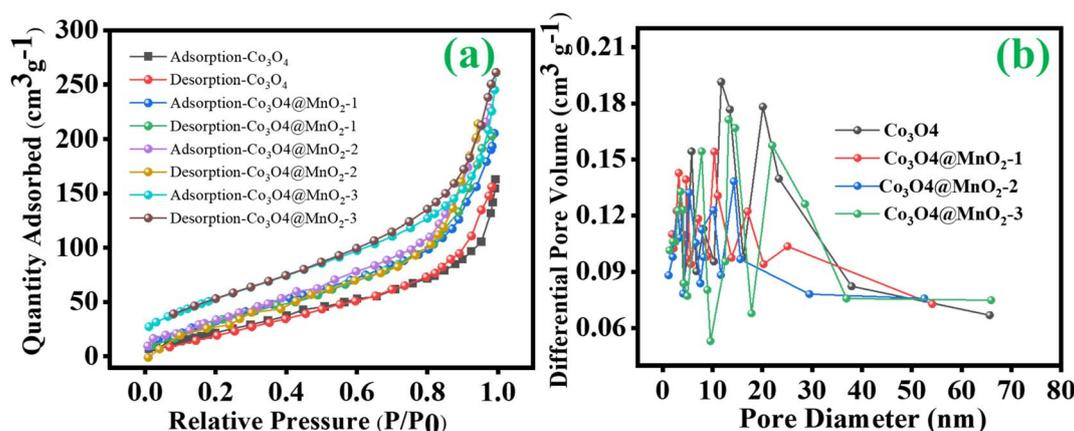
Fig. 5 (a) BET analysis and (b) BJH pore size distribution curves of ZIF-67 derived  $\text{Co}_3\text{O}_4$ ,  $\text{Co}_3\text{O}_4@\text{MnO}_2-1$ ,  $\text{Co}_3\text{O}_4@\text{MnO}_2-2$  and  $\text{Co}_3\text{O}_4@\text{MnO}_2-3$ .
