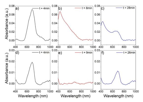
Fig. 8 Analysis of the absorbance spectra of thin layers of  $(C_4Py)_2[Ni_{0.5}Zn_{0.5}Zl_4]$  on glass used as gas sensors which were exposed in sequence to different gas mixtures: first, the gas sensors were exposed to a pure stream of dry  $N_2$  (0–5 min, (a and d)). Afterwards, ammonia vapor (b) or water vapor (wet  $N_2$ , (e)) was mixed to the nitrogen stream (5–10 min). Finally, the gas sensors were again exposed to a stream of pure dry  $N_2$  (c and f).
