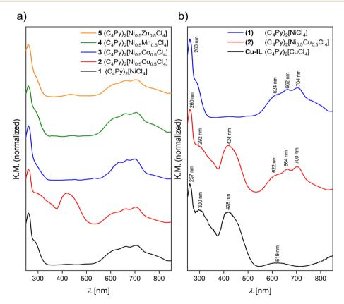
Fig. 7 (a) UV-Vis reflectance spectra of the Ni-containing ILs 1–5, (b) comparison of the UV-Vis spectra of the two ILs based on Cu only and Ni only,  $(C_4Py)_2[CuCl_4]$  and  $(C_4Py)_2[NiCl_4]$ , respectively, with the UV-Vis spectrum of the mixed compound  $(C_4Py)_2[Ni_{0.5}Cu_{0.5}Cl_4]$ , IL 2.
