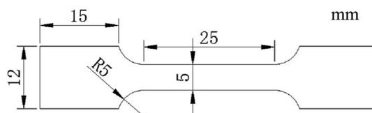
Fig. 2 Diagram of a tensile specimen.
