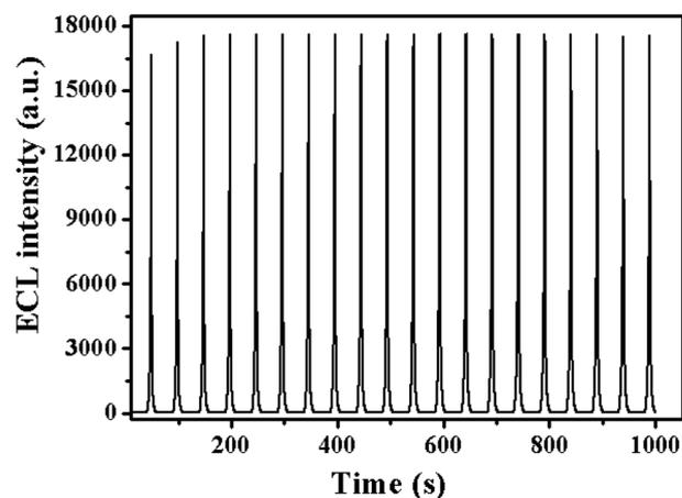
Fig. 3 ECL emission from the AuNPs/ $\text{NaBiF}_4 : \text{Yb}^{3+}/\text{Er}^{3+}$  UCNPs/GCE electrode in 0.1 M PBS (pH 7.4) containing 0.1 M  $\text{K}_2\text{S}_2\text{O}_8$  under continuous cyclic voltammetry for 20 cycles (scan rate: 100  $\text{mV s}^{-1}$ ; PMT voltage: 800 V).
