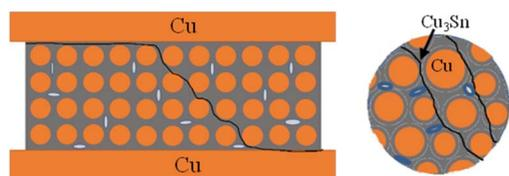
Fig. 12 Schematic diagram of fracture path of the joints of Cu/Cu<sub>3</sub>Sn/Cu.
