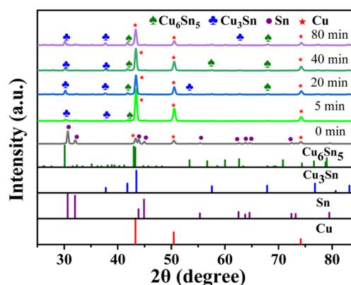
Fig. 5 XRD results of Cu@Sn preform after heating at  $280^\circ\text{C}$  for different holding time. Interfacial Structure Analysis of Cu@Sn Preform/DBC Substrate.
