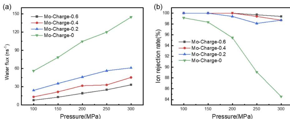
Fig. 6 BiMoS<sub>2</sub> water flux and ion repulsion for different charges. (a) Water flux and (b) ion repulsion rate as a function of applied pressure of BiMoS<sub>2</sub> nanopores.
