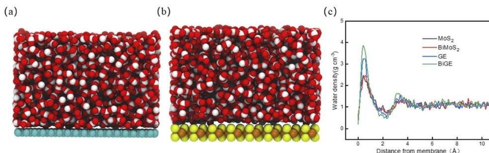
Fig. 2 (a) Snapshot of water on GE surface. (b) Snapshot of water on MoS<sub>2</sub> surface. (c) Mass density profiles of water molecules with the distance from nanosheets.
