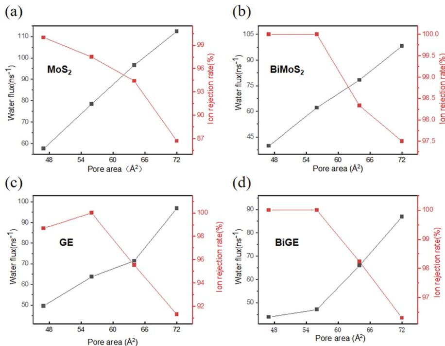
Fig. 3 Water flux and ion rejection against pore size of four membranes. (a) MoS<sub>2</sub> monolayer, (b) MoS<sub>2</sub> bilayer, (c) GE monolayer, (d) GE bilayer.
