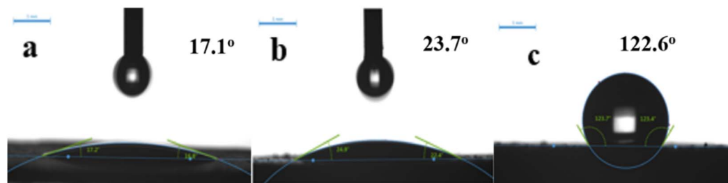
Fig. 8 Contact angle variation on (a) HZSM-5, (b) HCl-HZSM-5 and (c) HCl-OTS-HZSM-5 zeolite.
