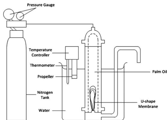
Fig. 4 Pressure driven dead-end filtration of laboratory-scale hollow fiber membrane for CPO refinery.<sup>2</sup>
