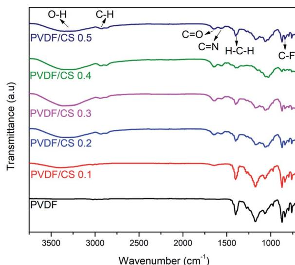
Fig. 6 Vibrational spectra of hollow fiber membranes.
