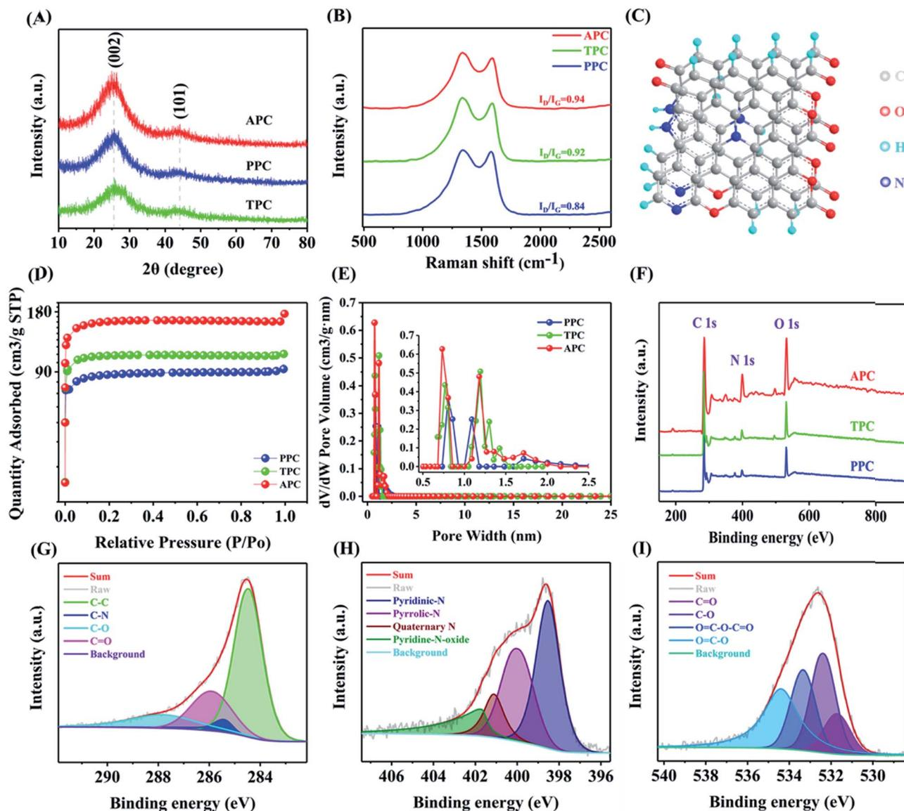
Fig. 2 (A) XRD patterns of APC, PPC, and TPC. (B) Raman spectra of APC, TPC, and PPC. (C) Molecular model of APC. (D)  $N_2$  adsorption/desorption isotherms of PPC, TPC, and APC. (E) Pore size distribution of PPC, TPC, and APC. (F) XPS survey spectra of APC, TPC, and PPC high-resolution spectrum of APC, TPC, and PPC. (G) C 1s, (H) N 1s, and (I) O 1s spectra of APC.
