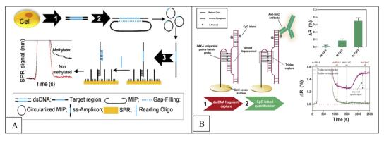
Fig. 4 (A) Methodological approach for the label-free and real-time detection of regional DNA methylation based on MIP and SPR.<sup>70</sup> (B) Scheme of the DNA methylation biosensor methodology.72
