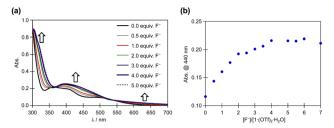
Fig. 6 (a) Family of absorption spectra collected during titration of a  $2.0 \times 10^{-5}$  M DMSO solution of  $1 \cdot (\text{OTf})_2 \cdot \text{H}_2\text{O}$  with a standard solution of TBAF. (b) Titration profiles at 440 nm.
