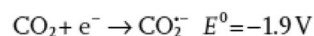
Fig. 1 Thermodynamic potential difference of the products made by the electrochemical reduction of carbon dioxide (CO 2 ). Reprinted with permission from ref. 31. Copyright 2016 Wiley.
