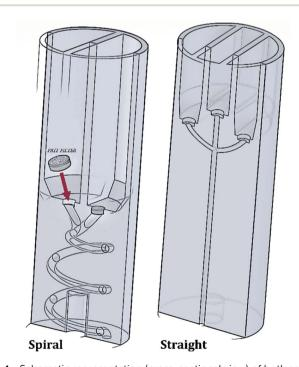
Fig. 1 Schematic representation (cross-sectional view) of both spiraland straight-RIAC prototypes. Both RIACs contain a recess at the bottom of each reservoir, to host a 3.175 mm steel HPLC-grade FRIT filter. The positioning of these filters is illustrated for the spiral-RIAC.
