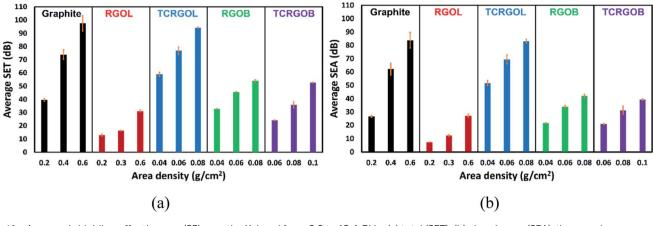
Fig. 12 Averaged shielding effectiveness (SE) over the X-band from 8.2 to 12.4 GHz: (a) total (SET), (b) absorbance (SEA), the error bars represent standard deviations.
