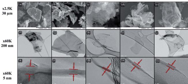
Fig. 5 SEM and TEM images of graphite and different RGOs. SEM images [30  $\mu$ m] (first raw): (a) graphite, (b) RGOL, (c) TCRGOL, (d) RGOB, and (e) TCRGOB. TEM images [200 nm] (second raw): (f) graphite, (g) RGOL, (h) TCRGOL, (i) RGOB, and (j) TCRGOB. TEM images [5 nm] for layer thickness identified with red arrows (third raw): (k) graphite, (l) RGOL, (m) TCRGOL, (n) RGOB, and (o) TCRGOB.
