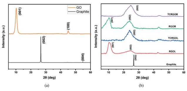
Fig. 6 XRD patterns: (a) graphite and graphene oxide (GO) and (b) graphite and different reduced graphene oxides.
