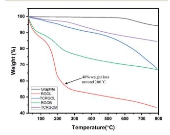
Fig. 7 Thermogravimetric analysis (TGA) for graphite and different reduced graphene oxides.
