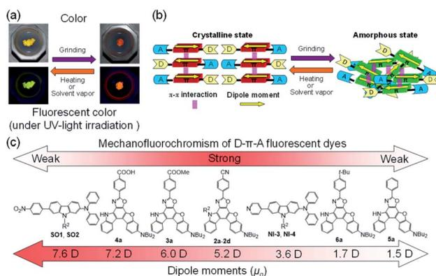
Fig. 1 (a) Photographs of powder of heteropolycyclic D- $\pi$ -A fluorescent dye under room light (top) and under UV-light irradiation (down) before and after grinding and after heating the ground solid. (b) Mechanisms of MFC observed in heteropolycyclic D- $\pi$ -A fluorescent dyes. (c) Correlation between dipole moments and MFC characteristics of D- $\pi$ -A fluorescent dyes.
