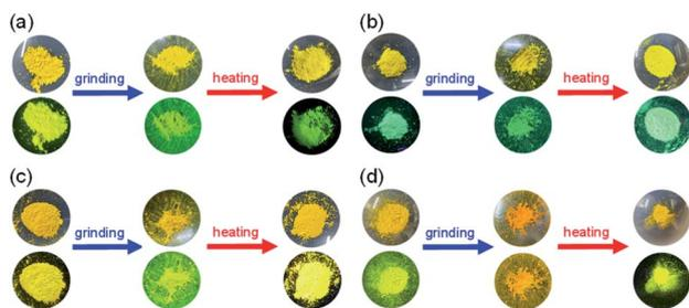
Fig. 5 Photographs of powder of (a) **OTK-2**, (b) **OUI-2**, (c) **OJK-2**, and (d) **OJ-2** under room light (top) and under UV-light irradiation (down) before and after grinding of as-prepared microcrystalline dyes and after heating the ground solids.
