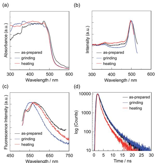
Fig. 8 (a) Solid-state UV-vis diffuse reflection-absorption, (b) fluorescence excitation at  $\lambda_{\text{max}}^{\text{fl-solid}}$ , and (c) fluorescence spectra ( $\lambda^{\text{ex}} = \lambda_{\text{max}}^{\text{ex-solid}}$ ) and (d) fluorescence decay profiles of OUK-2 before (as-prepared) and after grinding and after heating the ground solid at 180 °C.
