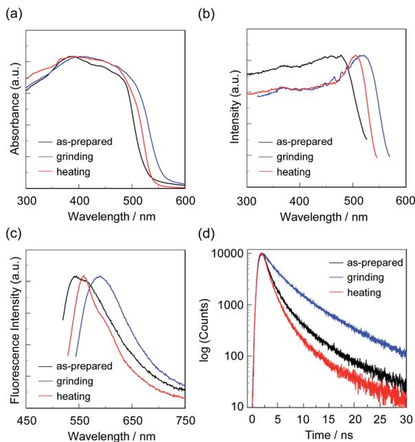
Fig. 9 (a) Solid-state UV-vis diffuse reflection-absorption, (b) fluorescence excitation at  $\lambda_{\text{max}}^{\text{fl-solid}}$ , and (c) fluorescence spectra ( $\lambda^{\text{ex}} = \lambda_{\text{max}}^{\text{ex-solid}}$ ) and (d) fluorescence decay profiles of OUJ-2 before (as-prepared) and after grinding and after heating the ground solid at 200 °C.
