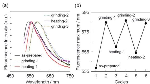
Fig. 10 (a) Solid-state fluorescence spectra ( $\lambda^{\text{ex}} = \lambda_{\max}^{\text{ex-solid}}$ ) of OUIJ-2 before (as-prepared) and after grinding and heating process. (b) Reversible switching of fluorescence maximum wavelength of OUIJ-2 during the grinding-heating process.
