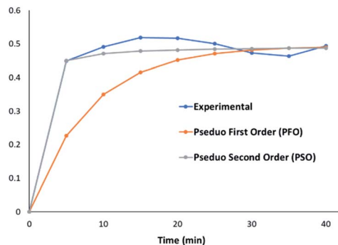
Fig. 5 Kinetic modelling for the adsorption of \text{MnO}_4^{2-} by 1 : 1 \text{CaCl}_2\text{DCGAC} in 0.00046 M \text{KMnO}_4 solution at room temperature.
