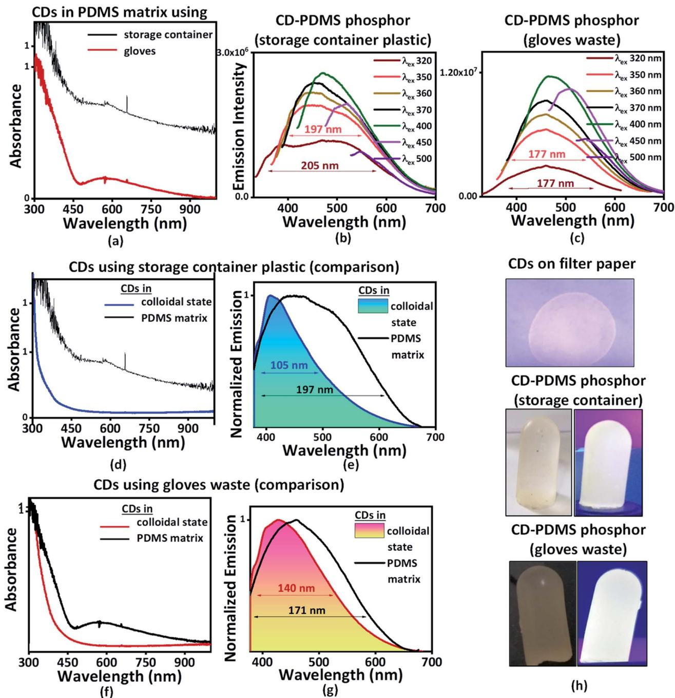
Fig. 5 Showing (a) absorption (b and c) emission spectra of plastic CDs in PDMS matrix. (d) Comparison between (d and f) absorption (e and g) emission spectra of plastic CDs in  $\text{CHCl}_3$  and in PDMS matrix. (h) Images (from top to bottom) of plastic CDs on filter paper under UV illumination, plastic CD PDMS phosphor (plastic CDs in PDMS matrix).
