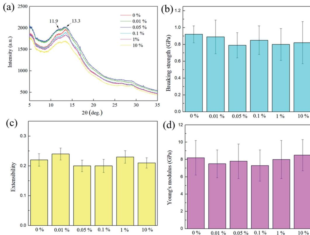
**Fig. 10** (a) XRD results for dragline silk modified with different aniline tetramer dip-coating concentration. Breaking strength (b), extensibility (c), and Young's modulus (d) are mechanical properties for dragline silk modified with different aniline tetramer dip-coating concentration. (Statistical analysis of breaking strength ( $P = 0.8942$ ), extensibility ( $P = 0.0579$ ), and Young's modulus ( $P = 0.9507$ ) revealed no significant differences among all aniline tetramer treatments).
