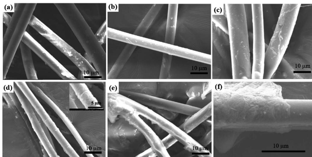
Fig. 5 SEM images of spider dragline silks modified with various concentration of aniline tetramer solution. (a) 0.01%; (b) 0.05%; (c) 0.1%; (d) 1%; (e) 10%; (f) 10%.
