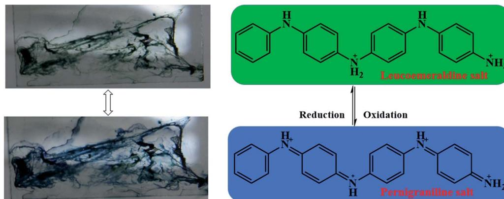
Fig. 8 Effect of applied voltage on the color of aniline tetramer/silk fibers (top: 0.1 V; bottom: 0.9 V). (dragline silk is modified with 1% of aniline tetramer solution).
