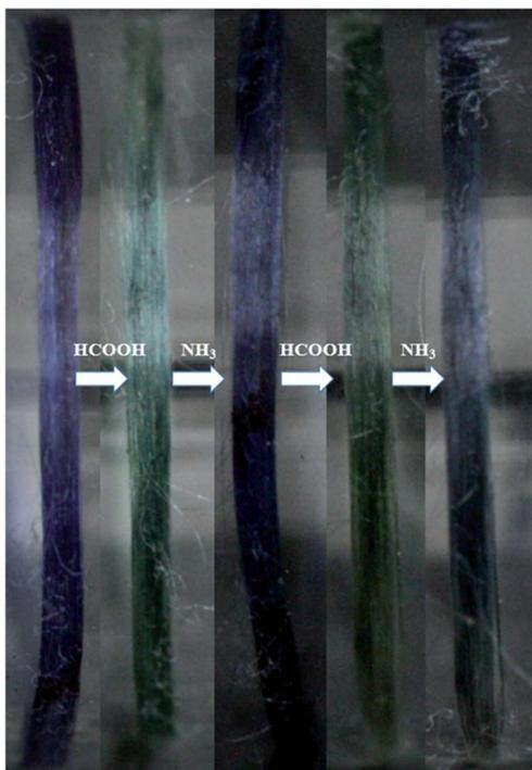
Fig. 6 Optical images of as-prepared aniline tetramer/dragline silk composite fibers cyclically exposed to formic acid (HCOOH) and ammonia (NH<sub>3</sub>) vapors. (Exposure time: HCOOH for 1 minute and NH<sub>3</sub> 10 minutes, respectively) (dragline silk is modified with 1% of aniline tetramer solution).
