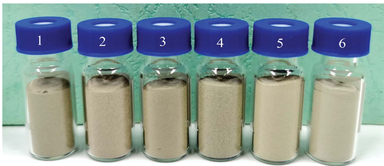
Fig. 6 Color comparison diagram of Fe-Co50@TiO 2 @Ag with the same Ag coating amount and different TiO 2 coating thicknesses (the feed ratio of TBT vs. Fe-Co50 is V_{\text{TBT}} : W_{\text{Fe-Co50}} = 1 : 3, 1.5 : 3, 2 : 3, 2.5 : 3, 3 : 3, and 3.5 : 3 ).
