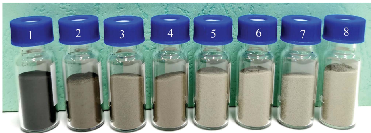
Fig. 5 Comparison of the Ag coating amount and the color of Fe-Co50@TiO 2 @Ag. No. 1 is Fe-Co50@TiO 2 before coating, and no 2–8 correspond to the following ratios of AgNO 3 vs. Fe-Co50@TiO 2 , W_{\text{AgNO}_3} : W_{\text{Fe-Co50@TiO}_2} = 0.4 : 10, 0.5 : 10, 0.6 : 10, 0.7 : 10, 0.8 : 10, 0.9 : 10, and 1 : 10 , respectively.
