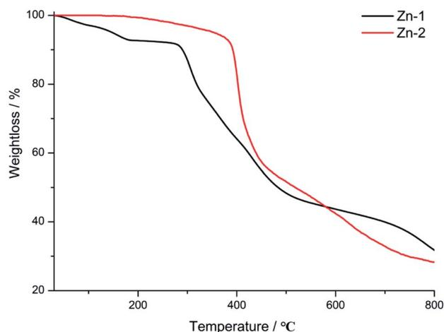
Fig. 3 Thermogravimetric curves of Zn-1 and Zn-2 in the temperature range of 30–800 °C under a N<sub>2</sub> atmosphere.
