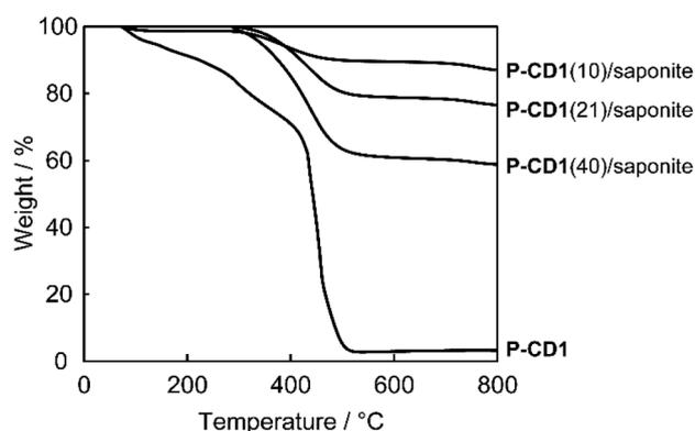
Fig. 2 TG curves of P-CD1 and the P-CD1/saponite composites with different ratios of CDs.
