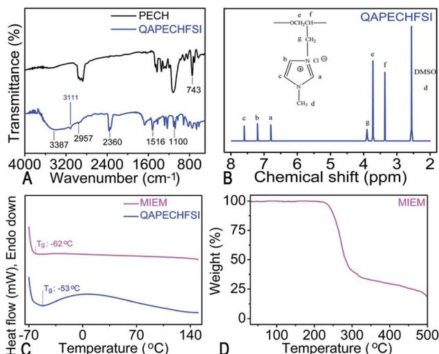
**Fig. 1** (A) Fourier-transform infrared (FTIR) spectra of the poly (epichlorohydrin) (PECH) and the quaternary ammonium poly (epichlorohydrin) with side chain of bis-(fluorosulfonyl) imide (QAPECHFSI); (B) <sup>1</sup>H NMR spectrum of the QAPECHFSI; (C) differential scanning calorimeter (DSC) curves of QAPECHFSI and the monolithic ionogel electrolyte membrane (MIEM); (D) thermogravimetric analysis (TGA) curves of MIEM.
