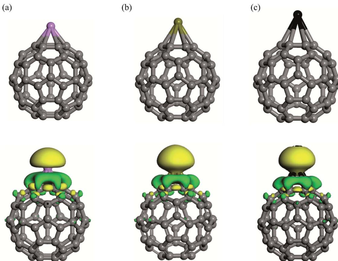
**Fig. 1** The relaxed structure (above) and EDR isosurface (below, isovalue =  $0.01 \text{ au}$ ) of (a) Li/ $C_{60}$ , (b) Na/ $C_{60}$  and (c) K/ $C_{60}$ . In the EDR isosurfaces, the gain and loss electron density areas are shown in green and yellow, respectively.
