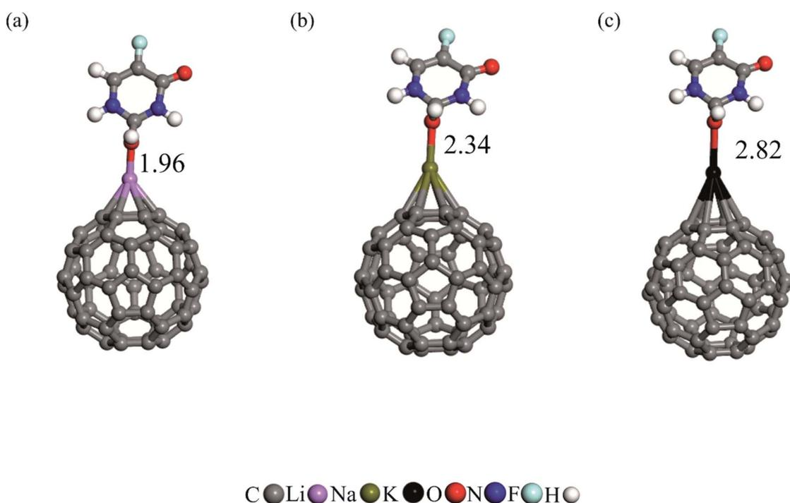
Fig. 5 The adsorption of protonated 5FU on (a) Li/C<sub>60</sub>, (b) Na/C<sub>60</sub> and (c) K/C<sub>60</sub>. All bond distances are in Å.
