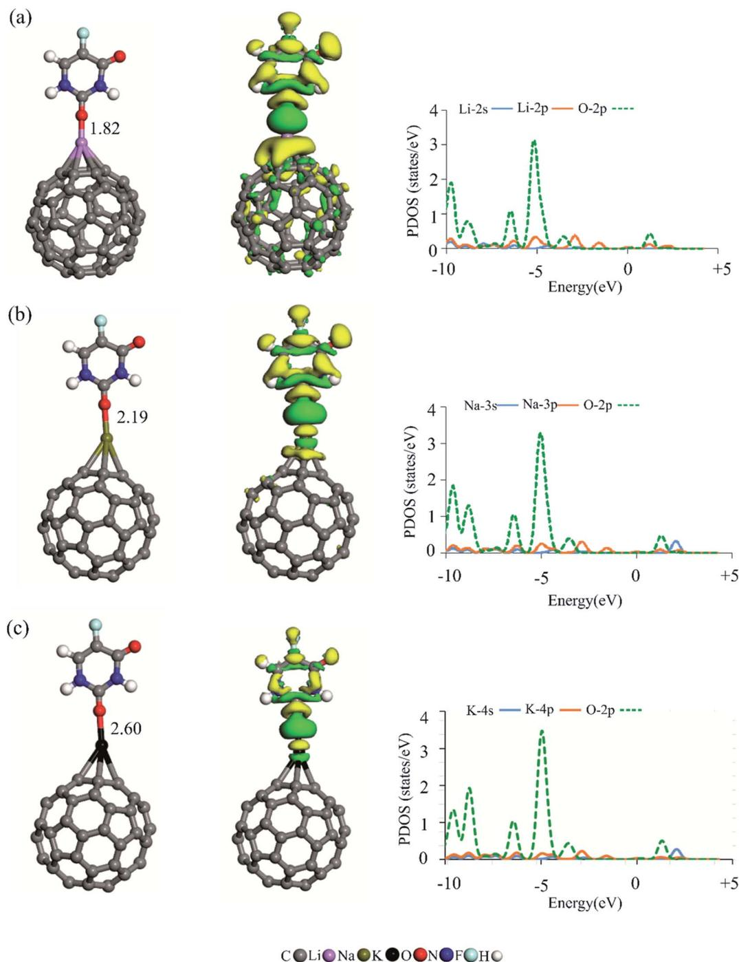
Fig. 3 The relaxed structure (left), corresponding EDR isosurface (middle, isovalue = 0.01 au) and PDOS plots (right) of the 5FU molecule adsorbed on (a)  $Li/C_{60}$ , (b)  $Na/C_{60}$  and (c)  $K/C_{60}$ . All bond distances are in Å. In the EDR isosurfaces, the gain and loss electron density areas are shown in green and yellow, respectively. The Fermi energy is set to zero in the PDOS plots.
