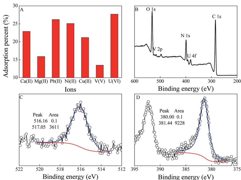
Fig. 5 Selective adsorption of U(vi) on PVPA/PAO (A).  $mV = 0.20$  g L<sup>-1</sup>, pH = 8.2 ± 0.1,  $T = 298 \pm 1$  K,  $C[\text{ions}]_{\text{initial}} = 50.0$  mg L<sup>-1</sup>,  $C[\text{NaCl}] = 0.10$  mol L<sup>-1</sup>, contact time: 24 h. XPS survey (B), V 2p (C), and U 4f (D) spectra of PVPA/PAO adsorbed U(vi) and V(v).
