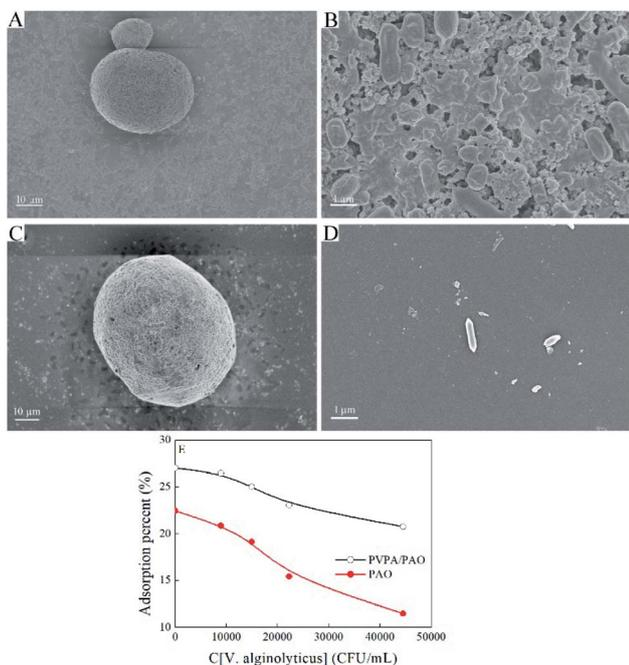
Fig. 6 SEM images of PAO (A, B) and PVPA/PAO (C, D) after adsorbing *V. alginolyticus* and U(VI), effect of *V. alginolyticus* concentration on the uptake of U(VI) by PAO and PVPA/PAO (E).  $T = 298 \pm 1 \text{ K}$ , contact time: 24 h,  $C[\text{U(VI)}]_{\text{initial}} = 50.0 \text{ mg L}^{-1}$ ,  $mV = 0.20 \text{ g L}^{-1}$ ,  $\text{pH} = 8.2 \pm 0.1$ ,  $C[\text{NaCl}] = 0.10 \text{ mol L}^{-1}$ .
